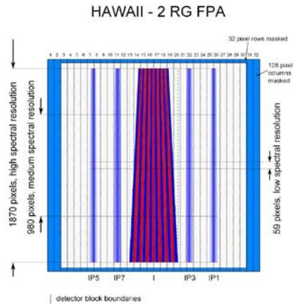
Figure 8: Interferometric and photometric beam configuration of the L band for R=500, and R=950.
