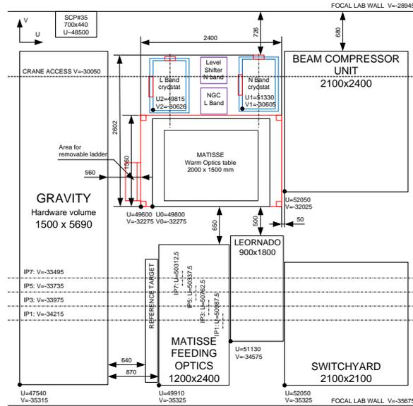
Figure 4: MATISSE, its Warm optics and the two cryostats housing the Colds Optics in the VLT interferometric laboratory.
