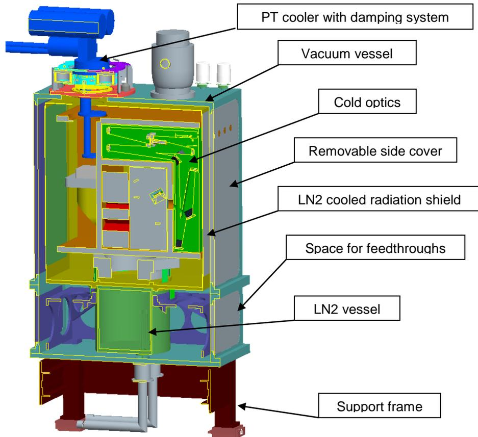
Figure 7: cross section through one MATISSE cryostat
