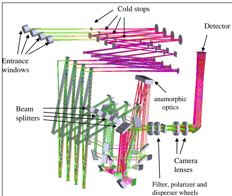
Figure 6: Layout of the interferometric light path
