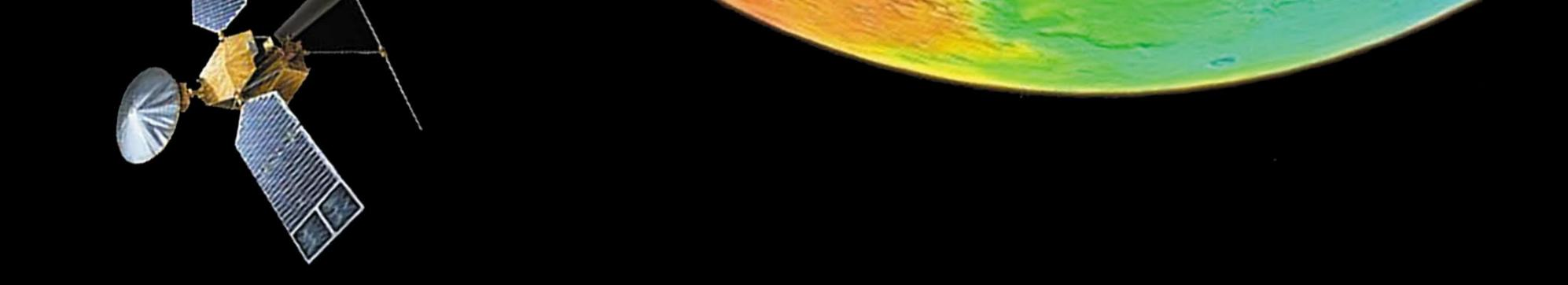
HiRISE (High-Resolution Imaging Science Experiment) flying aboard NASA's Mars Reconnaissance Orbiter (MRO) is the largest telescopic instrument ever sent beyond Earth's orbit and has been an indispensable instrument to help in the selection of landing sites on Mars.
