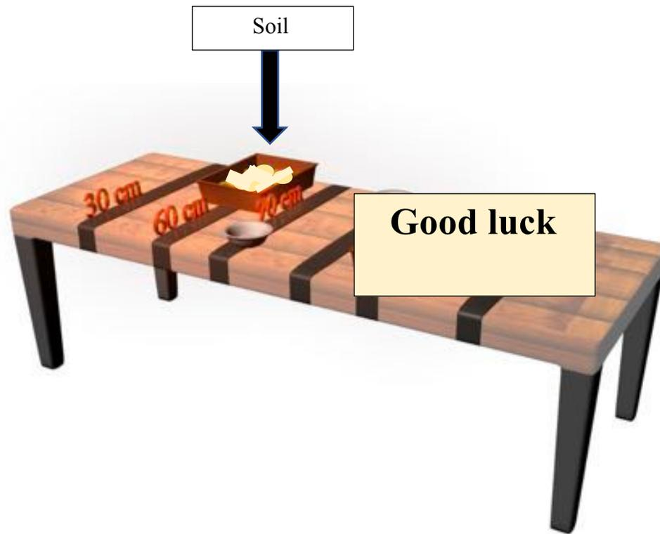
*Representation of a long table with two strategic locations for the shovel arm challenge. The goal is to use a student-designed robotic arm to move dirt / sand from the rectangular container (60cm line) to a container placed at the 70cm line without any part of the body sticking out the line of 30 cm.*
